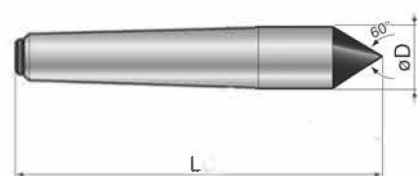
Hartmetallkopf Full carbide tip
